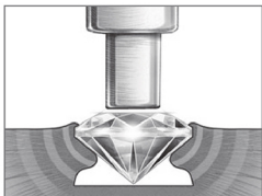
4 As the heated stone begins to melt the plastic material, the heating unit is used to push the stone gently down into that material.
