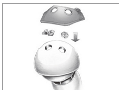
1 Here is an illustration of an earphone with three stones being put into place between the two layers of plastic.
