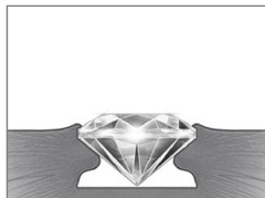
5 The heating unit is removed, and the stone and setting left to cool. The plastic now firmly holds the stone, just like a bezel.
