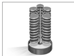
3 All the wax models are soldered on the so-called wax tree.
