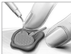
2 A vacuum needle is then used to mount stones by hand onto each of the wax models.
