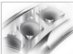
4 Next, the prongs are milled out of the metal part.
